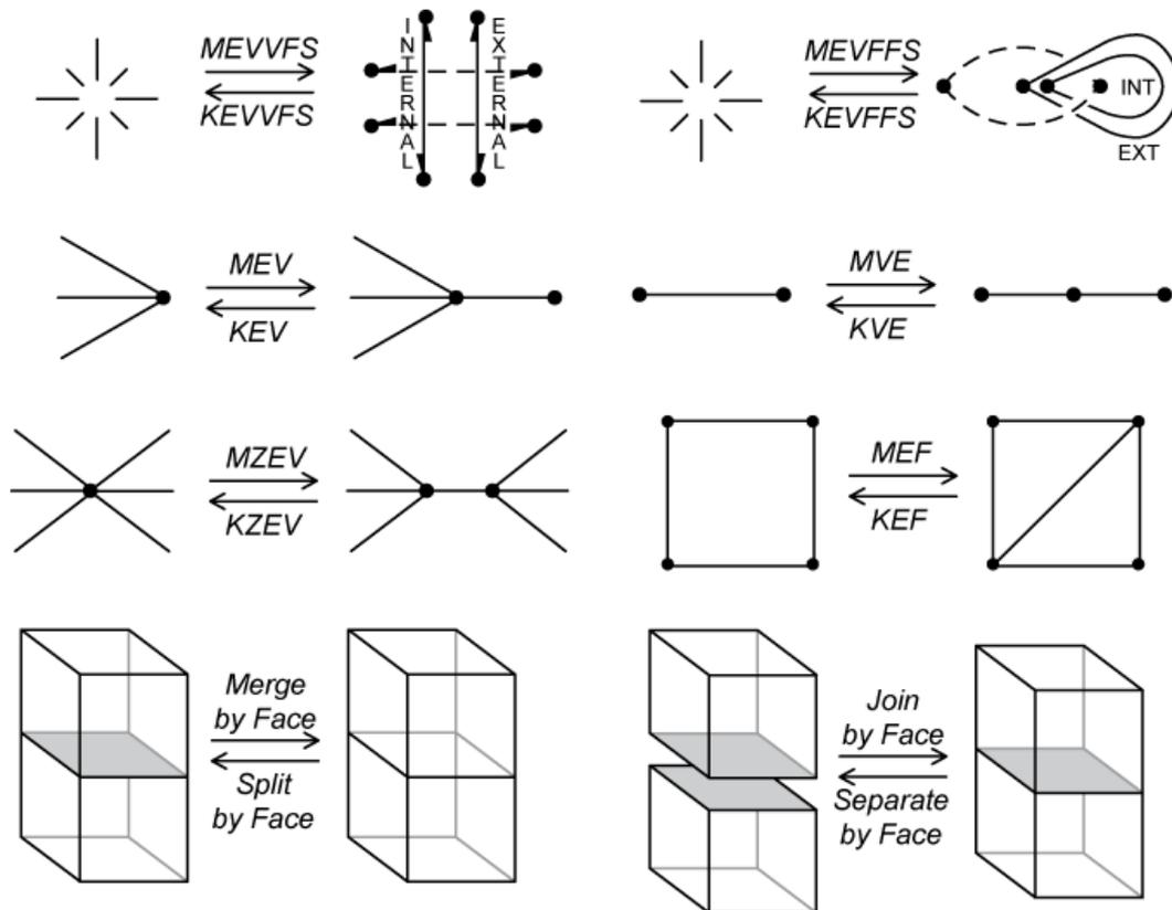
Figure 3: Euler operators and extended Euler operators (the dual and external part is shown only in a case of MEVVFS and MEVFFS).
