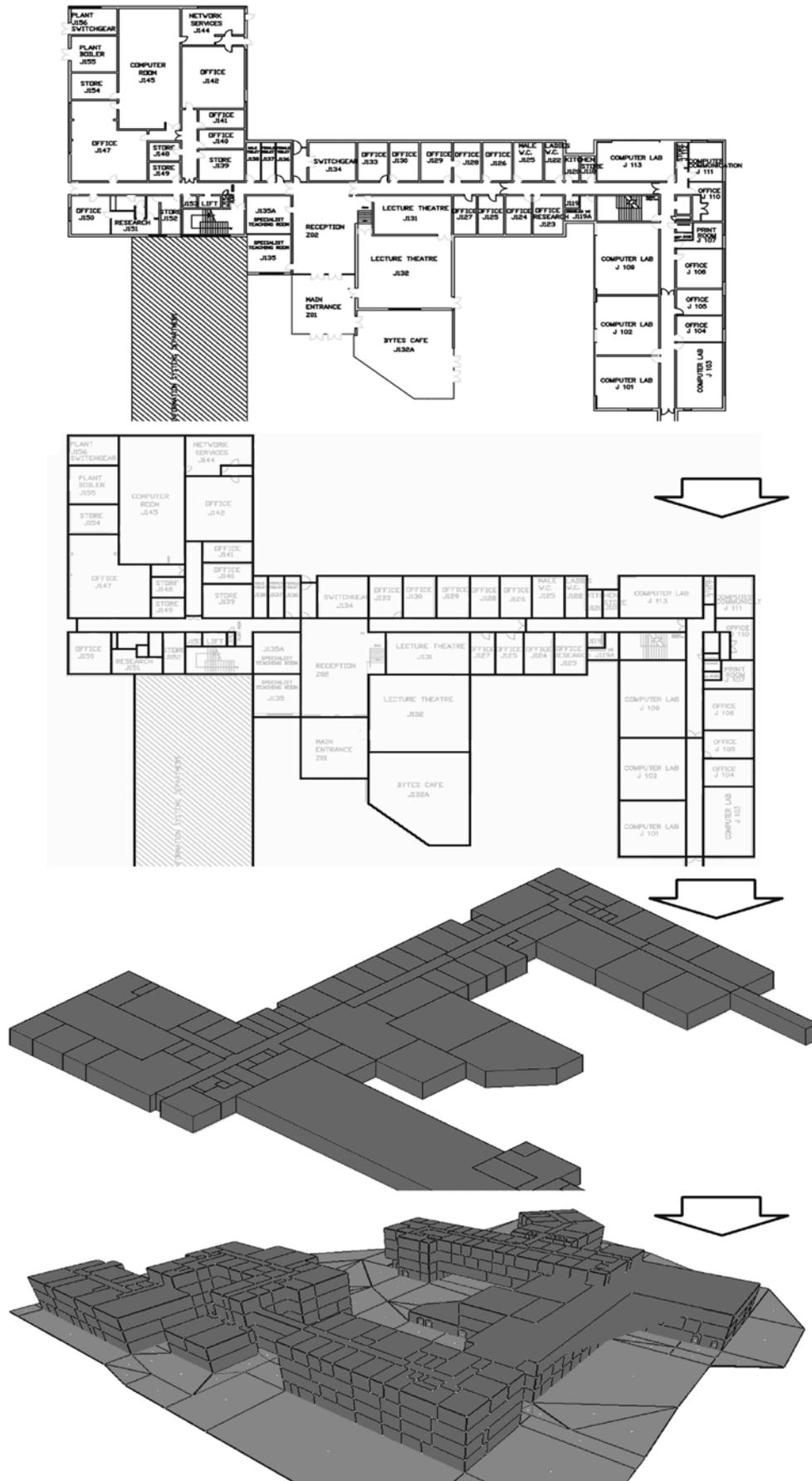
Figure 5: A 3D model reconstructed from paper plans.
