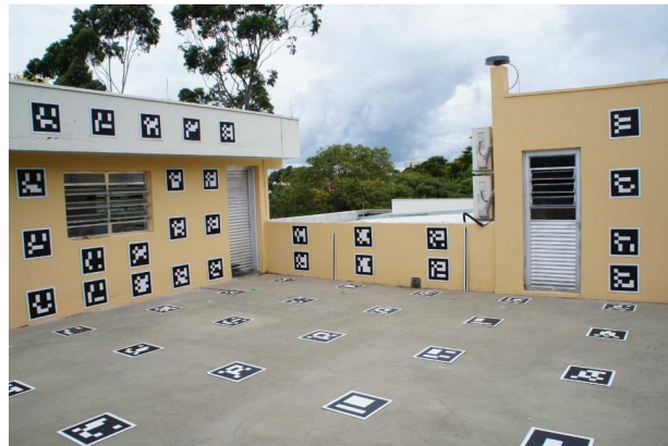
Figure 1. Terrestrial calibration field composed of Aruco coded targets.
