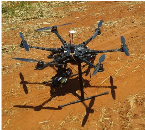
Figure 2. Hexacopter used to acquire the tropical forest images.
