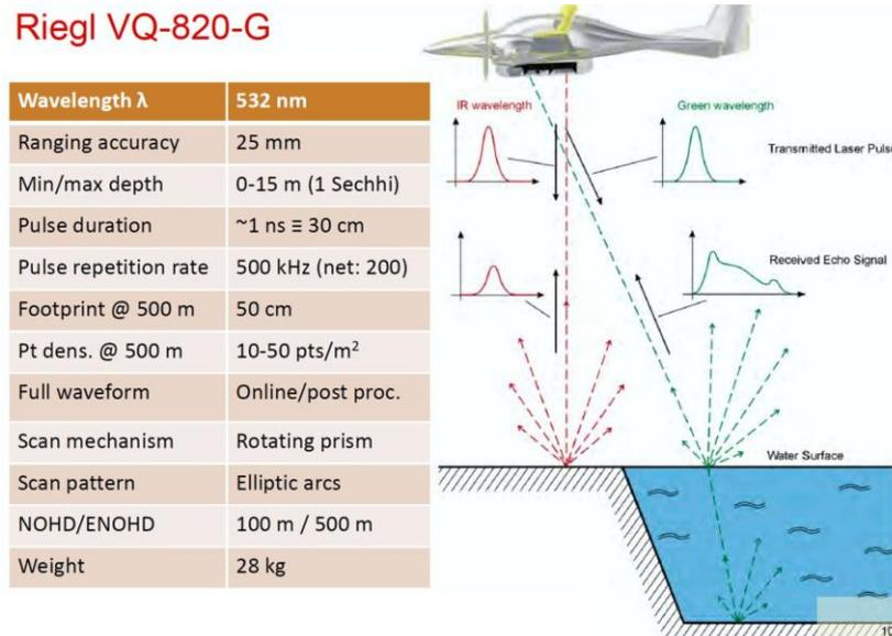
Fig. 8 Technical specifications of RIEGL VQ-820-G Topo-Hydrographic Airborne Laser Scanner with a scheme of the reflecting signal from underwater ground object
