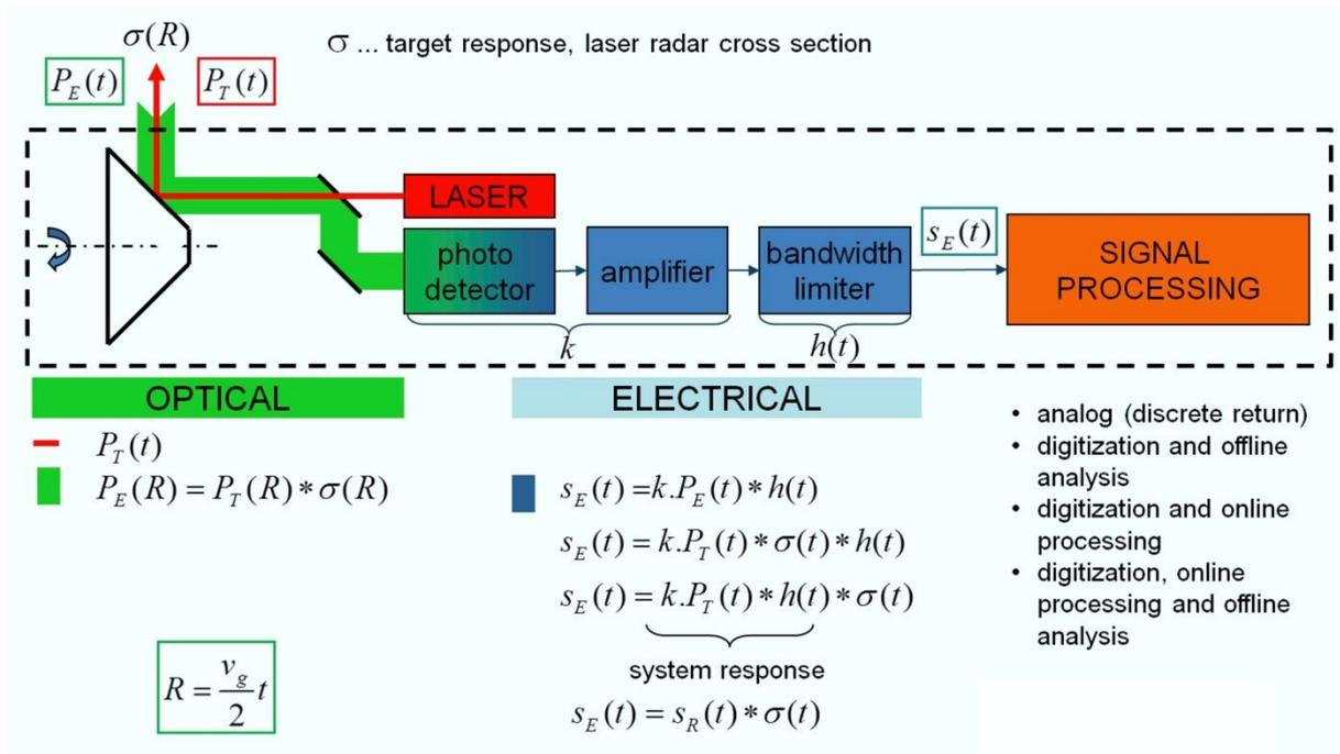
Fig. 2 Block diagram of RIEGL LiDAR instrument
