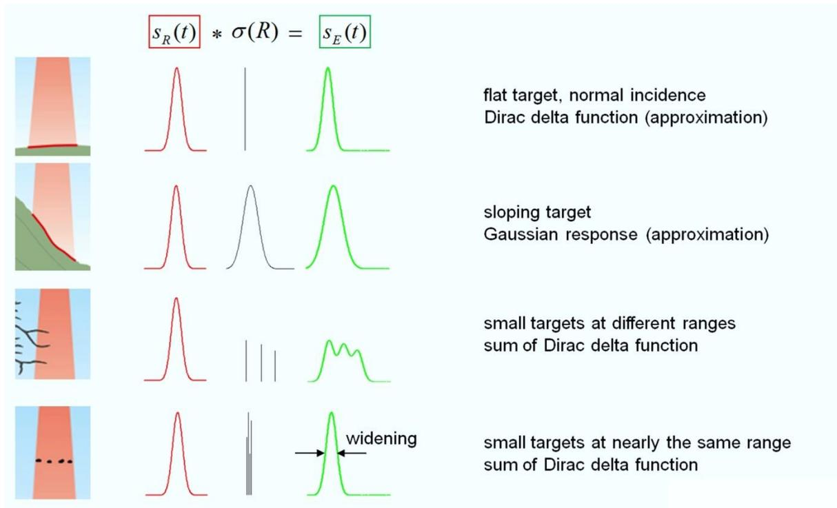
Fig. 4 Amplitude comparison received from the various objects
