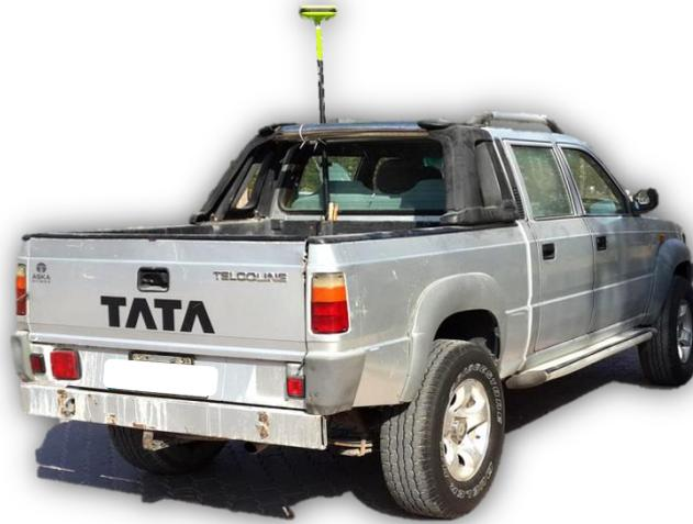
Figure 4 Receiver (Rover) Located on the Car
