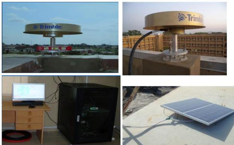
**Figure 1:** State-of-the-Art GNSS CORS Infrastructure in Nigeria (Ojigi et al, 2011)
