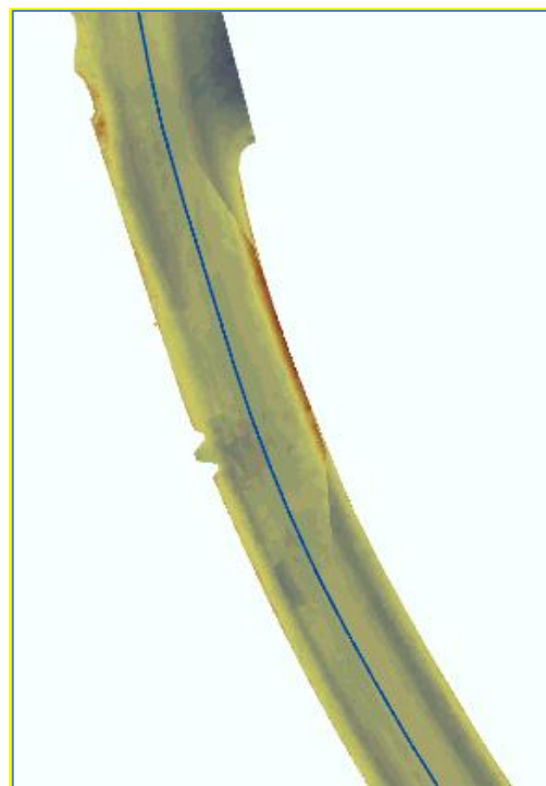
Figure 3 An example of water depth differences using catalogued measures. The different colours indicate different water depths differences. Red shows shortage and blue shows surplus in meeting the minimum water depth requirement.
