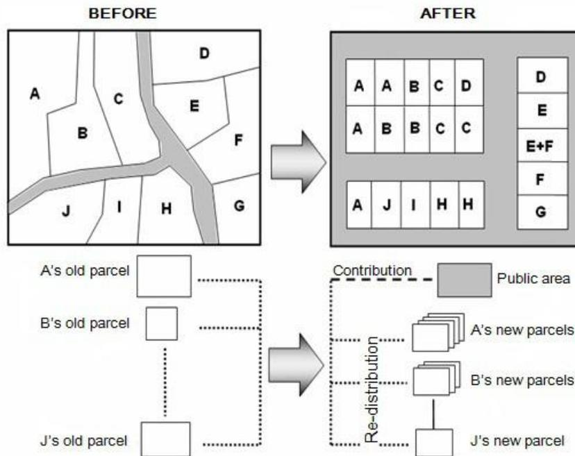
Fig. 1. Mechanism of LR (Yomralioglu, 1993).
